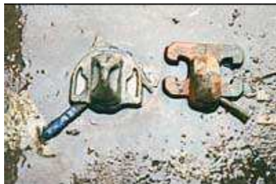
Photo 3 - Perennial problem of left-hand & right-hand locking twistlocks, which occurring on the same ship can undermine the integrity of the securing arrangement.
